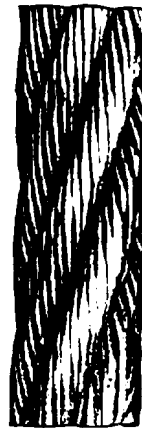
Figure 4-42. Effects of Abrasion and Peening
