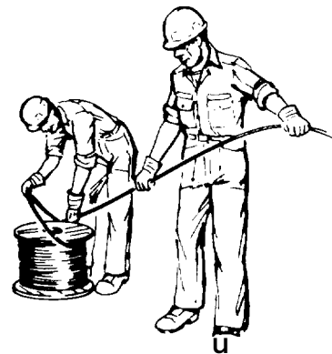
Figure 4-28. Incorrect Method of Uncoiling Wire Rope
