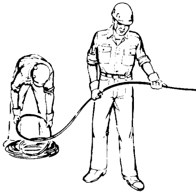
Figure 4-27. Incorrect Method of Unreeling Wire Rope
